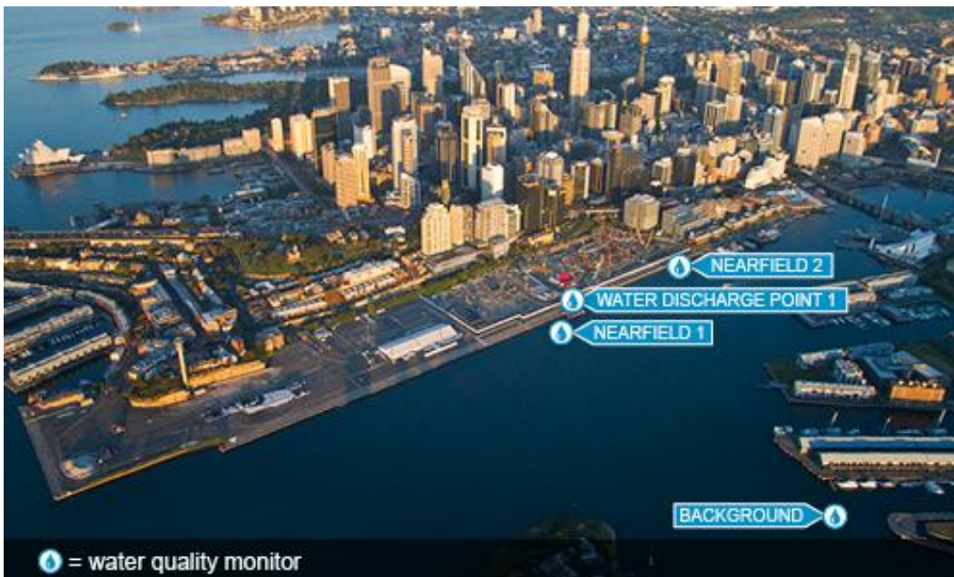
Approximate locations of water monitoring equipment
