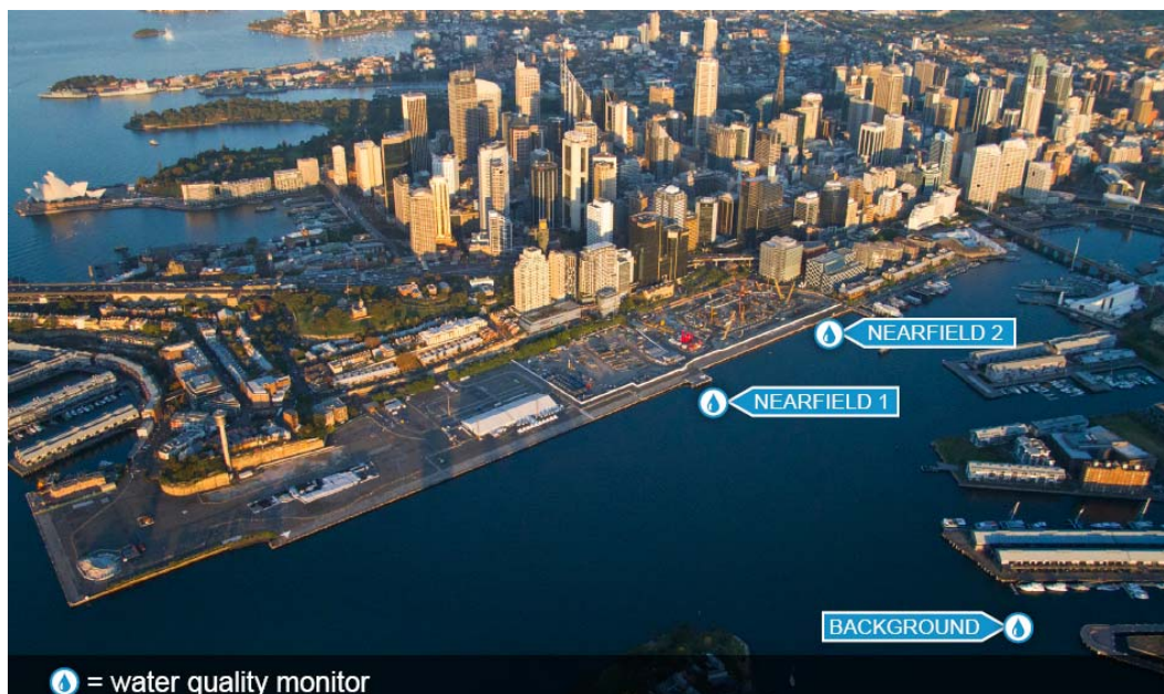
Approximate locations of water monitoring equipment
